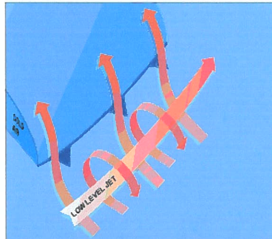
Fig. 2-8 - Complex winds around low-level jet: can result in significant wind shear and turbulence
